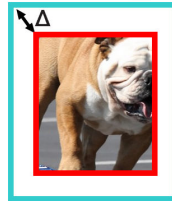
Figure 3.2: An example of bounding box regression, the detected box (red) is misplaced and does not match the correct one (blue), we hope that the network can recognise that the object detected (dog) is missing some of its parts and outputs (i.e. the regressor) an offset \Delta(x, y, w, h) to correct the predicted box.
